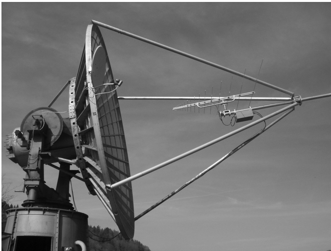
Fig. 5. Picture of the 5m dish at Bleien with the low-frequency-antenna pointing to the mirror
