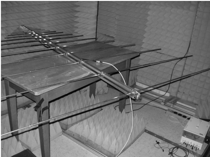
Fig. 7. The low-frequency-antenna in the absorber room at ETH-ETZ
