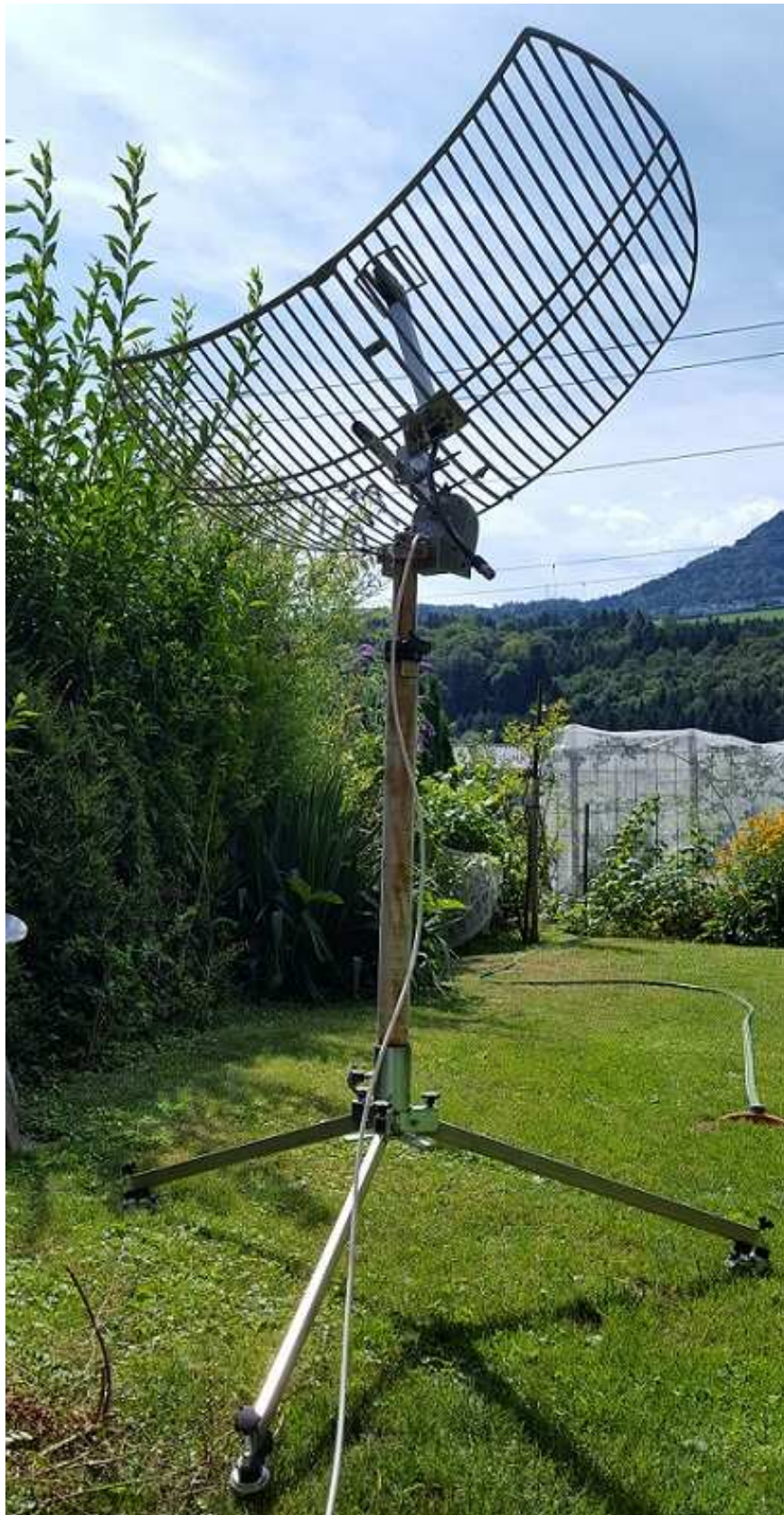
Fig. 8: S-band antenna with Sat-rotor on a tripod tracking the Sun.
