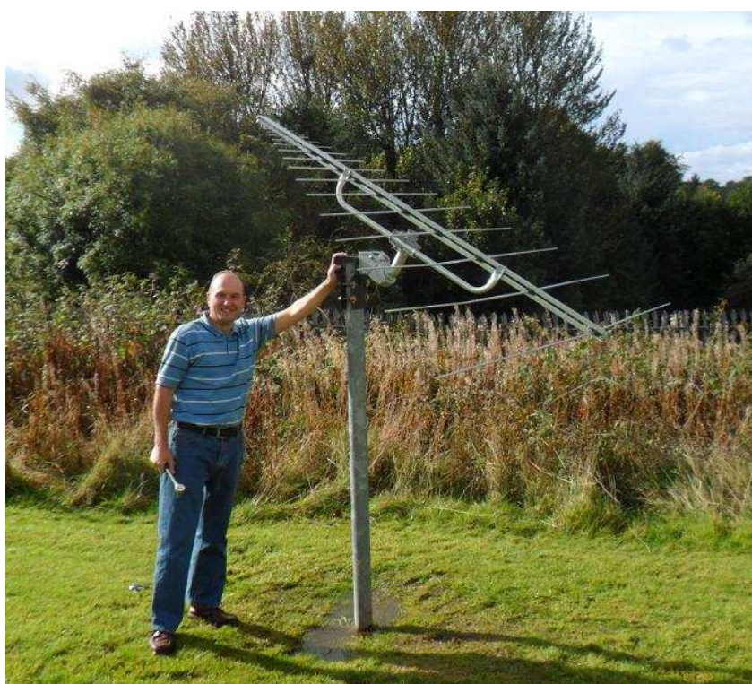
Fig. 4: How to install SAT-rotor for pseudo parallactic mount with tracking in local hour angle only at fixed declination. Depending on mounting method the command for hour angle needs to be changed from ha to -ha.
