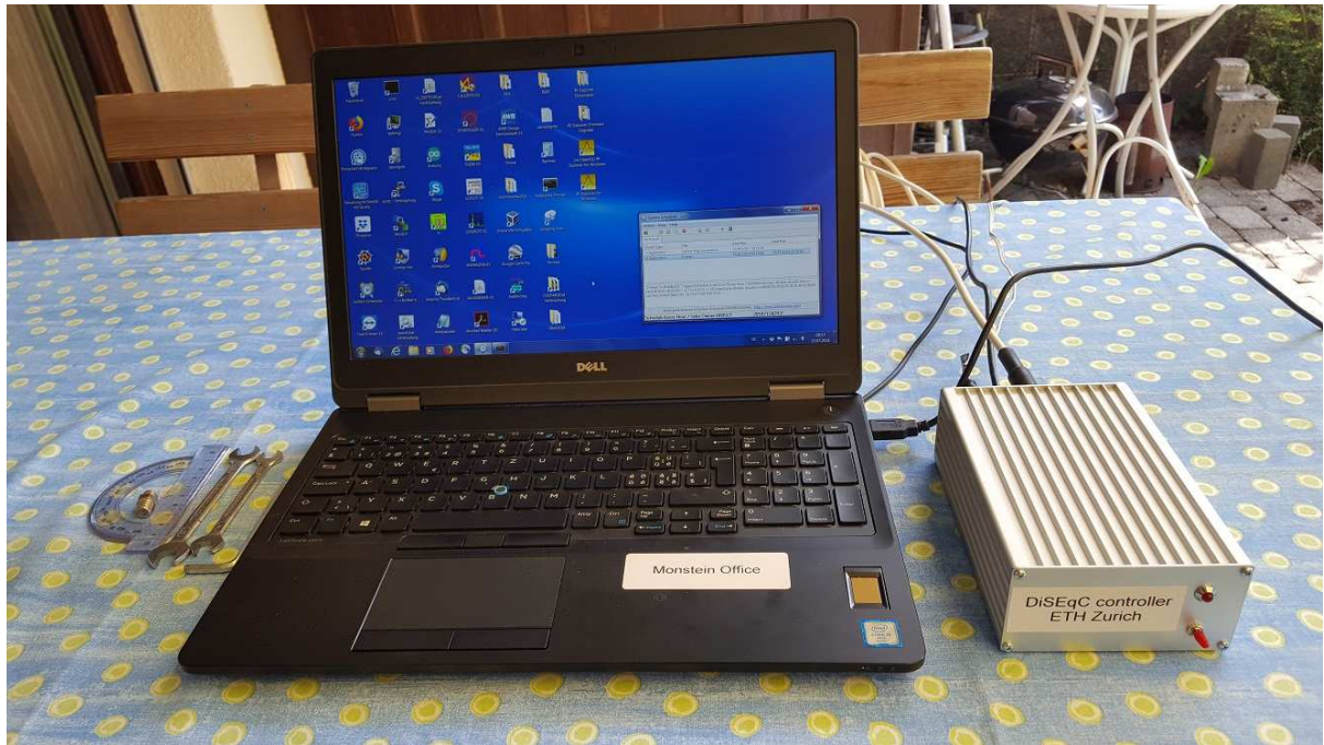
Fig. 7: Control PC and rotor controller box. A Python script is called every 5 minutes and commands the rotor to the actual Sun position.
