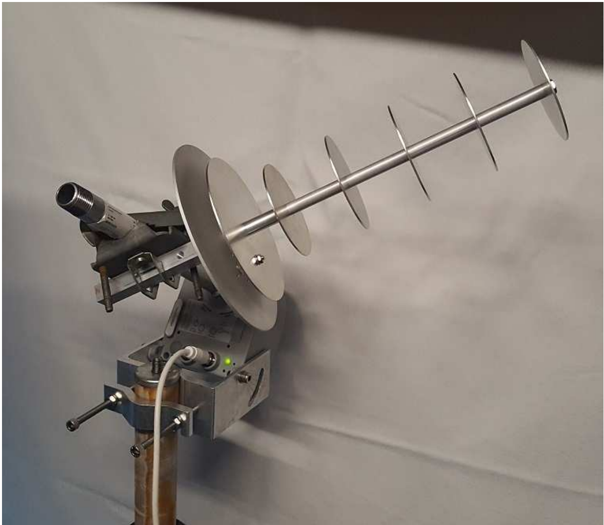
Fig. 5: Simple rotor with a shaft extension by a piece of water pipe 1/2". For demonstration a small L-band antenna has been attached.
