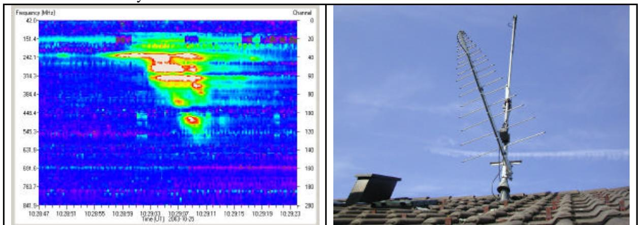
A bright solar flare from last Saturday was captured with my home test setup (1 CALLISTO receiver connected to a standard PC). Although the antenna on top of the roof (see above right) is only an amateur log-per, the signal/noise is rather good due to strong flux values (200sfu at 203MHz and 5400sfu at 410MHz according to <http://www.sec.noaa.gov/ftpd/indices/events/20031025events.txt>).
