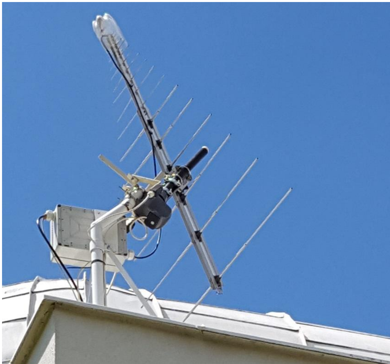
Fig. 2: LPDA with Suntracker at Hurbanovo observatory, Slovakia. Declination is changed manually about once a month.
