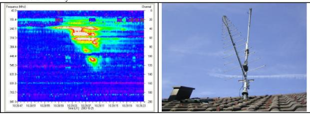
A bright solar flare from last Saturday was captured with my home test setup (1 CALLISTO receiver connected to a standard PC). Although the antenna on top of the roof (see above right) is only an amateur log-per, the signal/noise is rather good due to strong flux values (200sfu at 203MHz and 5400sfu at 410MHz according to <a href="http://www.sec.noaa.gov/ftpdir/indices/events/20031025events.txt">http://www.sec.noaa.gov/ftpdir/indices/events/20031025events.txt</a>).
