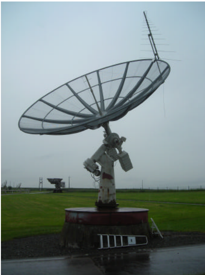
Figure 1: Remaining interferometer antenna at Humain station of ROB with broad band antenna attached to the rim of the dish. The dish with its mount and drives is only used as a positioning tool for the broad band antenna. In the background one can recognize an old "Würzburg Riese" from World War II. The logarithmic periodic antenna CLP-5130-1N covers the frequency range of 50MHz up to 1300MHz. While Callisto in most cases only makes use of a part of the spectrum, in this case. 45 MHz - 90 MHz as presented in figure 3.
