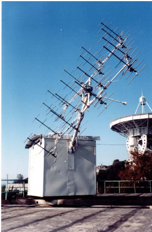
Fig. 2: Left: Phased array of 16 elements (4x4) with total size of 3.5x3.5 meter. Every element consists of 7 dipoles each. The frequency range is 250-350 MHz; the beam pattern is of order of 11^\circ . The aerial is fixed on a parallactic mount with an electric drive to track the sun from 5 UT up to 13 UT. Preamplifier is a ZX60-33LN+ having a gain of 20 dB (placed in antenna box). Coaxial cable is 40 meters long with a loss of about 4 dB.
