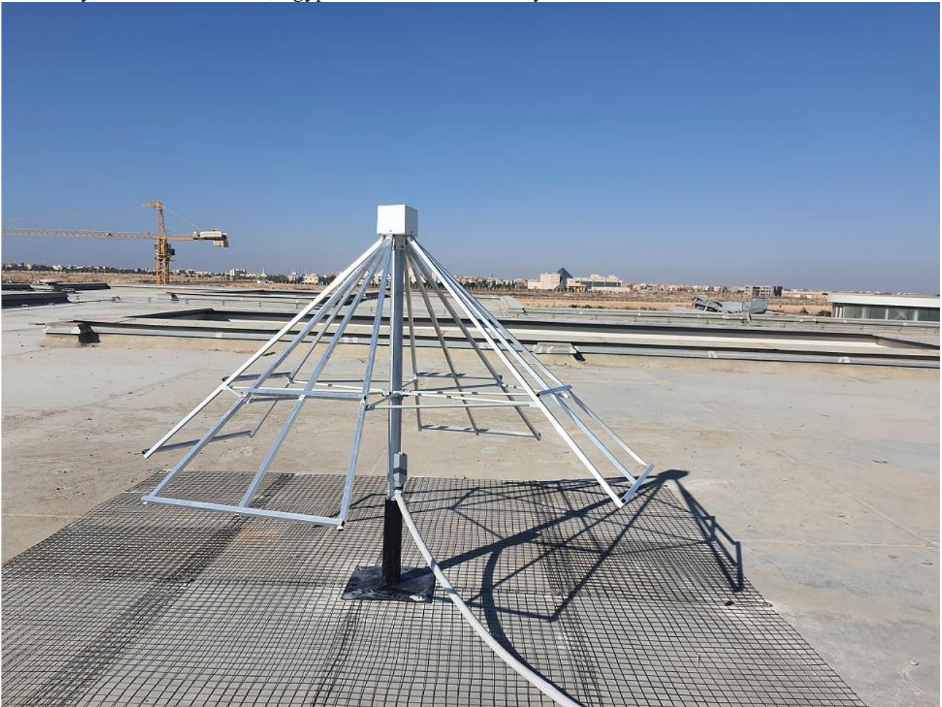
Fig. 1: LWA on the roof of the University with ground mesh to improve beam pattern. Frequency range 10 MHz - 80 MHz.
