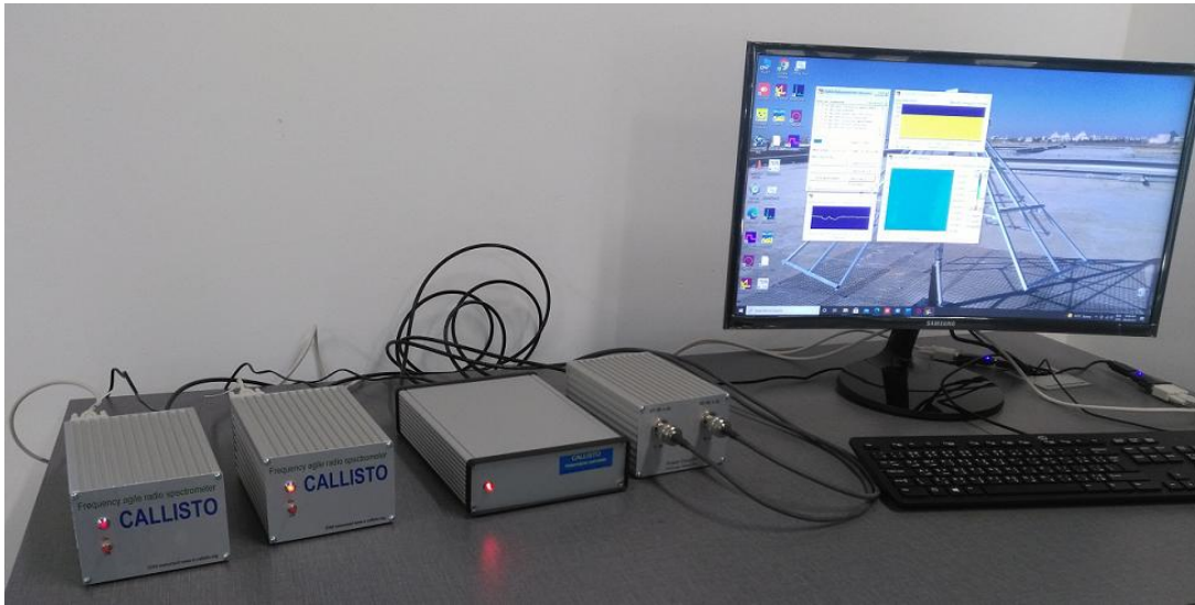
Fig. 2: From left to right: 2 spectrometer CALLISTO, dual channel heterodyne up-converter, power supply and 90° quadrature hybrid to convert linear polarization into circular polarization, PC.
