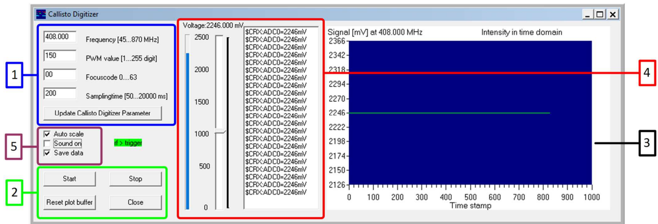
Figure 5 ~ Digitizer window. In this example, the right frame is displaying measurements at the log detector output in mV for a 408.0 MHz input signal with a level of -70 dBm from an RF signal generator. The thin green trace shows the steady signal at 2246 mV that has progressed about 800 seconds in the 1000 second wide window. The middle (red) frame shows the actual measured values at 200 ms intervals. See text.
