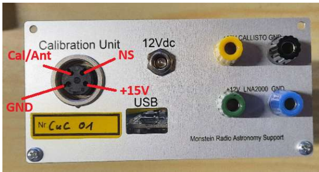
Fig. 6: Backside of CuC with connectors for Calu, Callisto, LNA, USB and 12v DC-power
