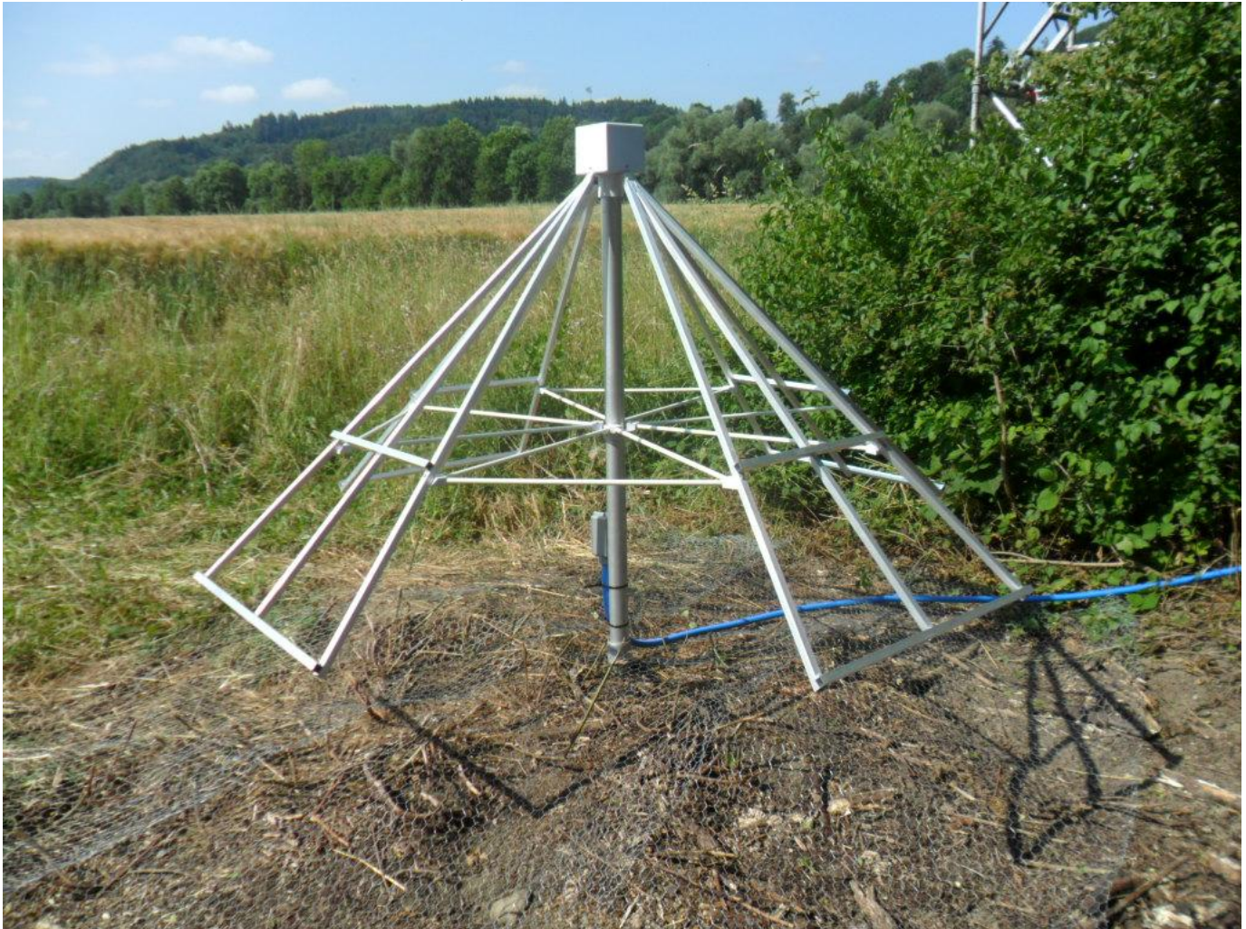
Figure 3 ~ LWA at Bleien observatory. Chicken wire mesh acts as a ground reflector. Currently only one polarization is operational. In the future it is planned to upgrade for a second polarization combined via a 90^\circ quadrature hybrid to get circular polarization LHCP and RHCP. This to test a new FFT-spectrometer in terms of SFDR, dynamic range, polarization cross-talk, sensitivity, stability etc. The antenna was installed by apprentice Alexander Zvyagin during his 3rd year educational exercises. Image by Chr. Monstein.
