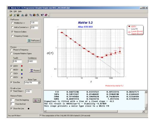
Figure 4: ALLAN-variance plot for Callisto at f = 610.0 MHz. The x-axis shows the integration time  $\tau$  expressed in seconds over an observation time of 6 hours and 3 minutes, the y-axis the variance  $\sigma$  of the signal, both in logarithmic scale.
