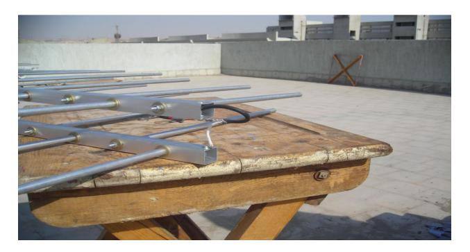
We should connect the the wires inside each boom in order not destroy form sun and weather conditions.
